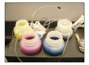
4. Take note of the coloured band on each of the colour ink lines, and match this to the ink in each of the containers when screwing the containers back in to the lids. To screw the containers to the lids, simply hold the lid firmly and screw the container up into the lid.
