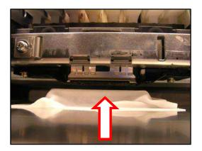
Do not allow the sponge to press too hard against the print head as this will cause catastrophic damage to the print head, carriage assembly and platen drive system. The sponge must be compressed to NO LESS than two thirds of its original height.
