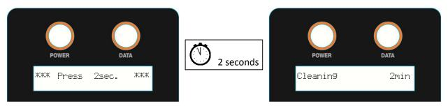
4. The operation panel will display the remaining time until the clean is finished. After about two minutes or so the clean operation will complete.
