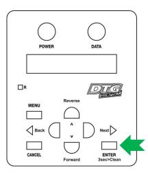
3. The operation panel will display \*\*\*\* Press 2sec. \*\*\*\* . After about 2 seconds the printer will begin head cleaning.
