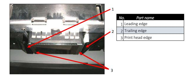
1. Carefully clean the metal edges of the print head with a swab and cleaning solution.
