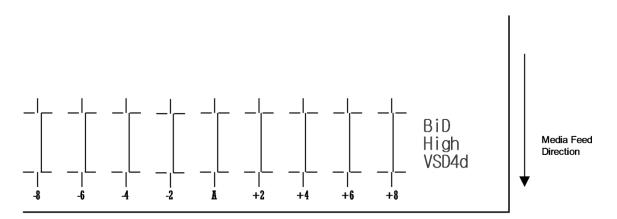
The objective is to have the centre vertical bar of the pattern marked "A" to align with the top and bottom shorter vertical bars. This is accomplished by applying an offset value (via the screen / keypad) to compensate for the difference between the printed position and the desired position:
