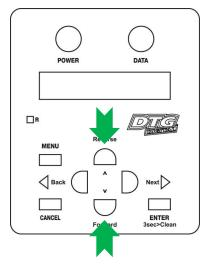
5. To save the changed setting, press the [Enter] key on the operation panel.
