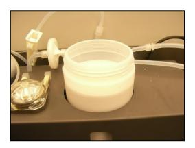
9. Now screw the container back up to the lid. To do this simply hold the lid firmly and screw the container up into the lid. Double check that all tube clamps are in the open position and all connectors are firmly joined.
