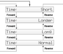
3. When the [Enter] key is pressed to confirm / select the Menu Cleaning menu option, the first item of the Cleaning Menu will display – Time: Short.
