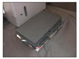
4. Carefully insert the rear of the platen into the Acu-Lok slot and ensure that the alignment pins are protruding correctly through the holes in the front of the platen bed.
