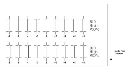
The printer will automatically align the successive prints correctly progressively down the page. NOTE
