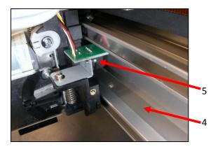
Using a microfibre cloth (as supplied in the maintenance kit of the printer), moistened with distilled or purified water, or approved Cleaning Solution, GENTLY rub both faces of the encoder strip.
