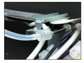
8. Draw on the syringe plunger to pull the ink through from the ink bottle towards the 3 way joint. Stop drawing when the ink reaches (approximately) the position indicated here:
