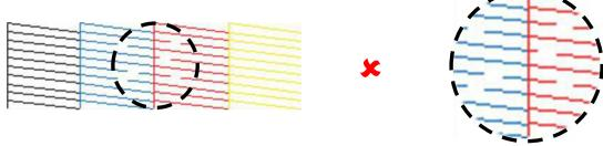
FIGURE 3-6 NOZZLE TEST PRINT - MISSING NOZZLES
