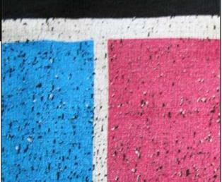
FIGURE 4-3 EXCESSIVE PRETREATMENT EXAMPLE
