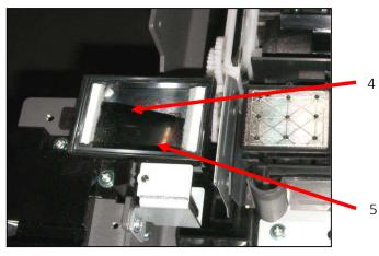
Do not allow the Carriage assembly to remain out of the capping station for longer than two or three minutes. Failure to do so will result in possible blockage of print nozzles due to ink drying. This may result in irreversible damage to the print head requiring print head replacement.
