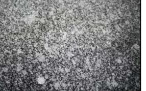
FIGURE 4-2 AN EXAMPLE OF INSUFFICIENT PRETREATMENT
