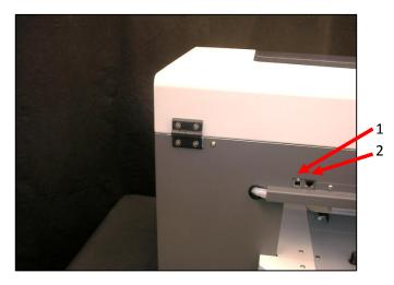
No.Part name1USB interface connector port2Network interface connector port
