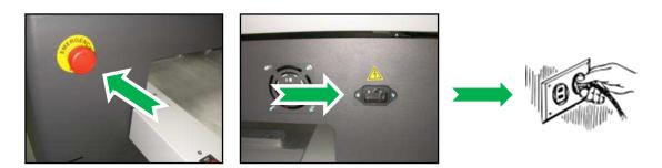
5. Rotate the red cap of the emergency stop to allow the printer to receive power.
