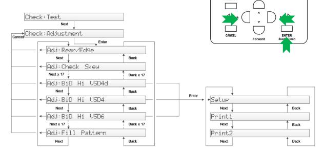
FIGURE 3-11 ADJUSTMENT MENU FLOW
