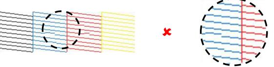
FIGURE 3-7 NOZZLE TEST PRINT - MISPLACED NOZZLES
