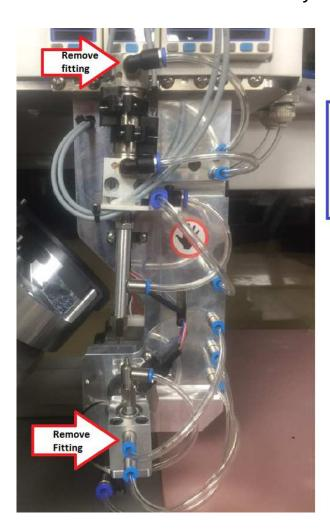
Twice a month you will want to remove the top fitting of the Swing gun and the top fitting of the Setter gun and place two drops of oil into the cylinder.
