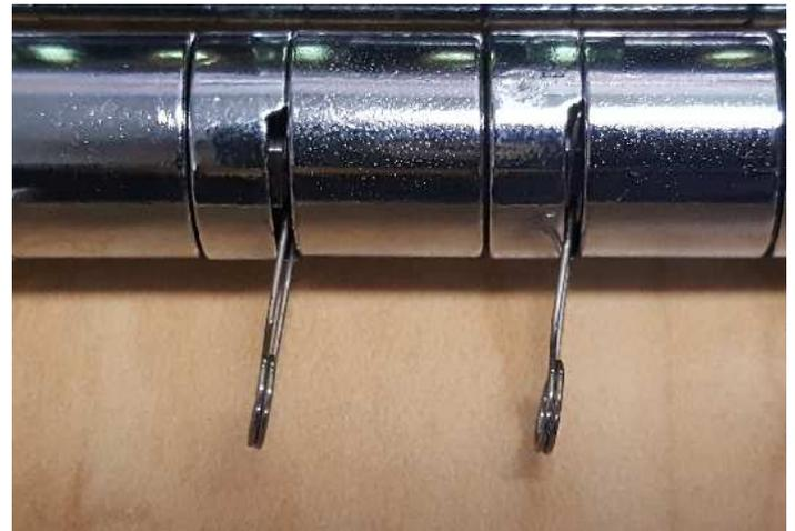
Once you have all the pieces and springs back in to place, place the holder on the left side as shown below and slide the bar assembly in on the right side. Then, line up the bar on the left and slide in to position.
