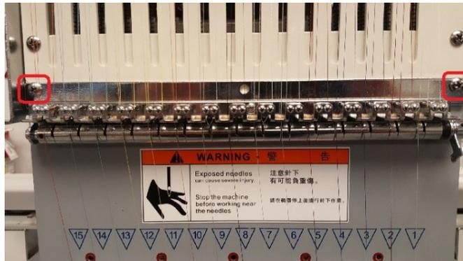
Next, lay the assembly on a flat surface and take a picture so you can put it back together the same way it was. Loosen the Allen screw holding the spring lever to the far right, so that you can remove it and set it to the side. Be careful with the spring holding the lever in place. It will pop the lever out at you and the spring could get lost. Hold the spring lever while loosening the screw, then pull them off together and set aside.
