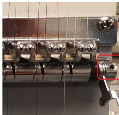
Lay the assembly on the flat surface with all the springs flat against the table. Loosen the two 1.5mm Allen screws on either end, so that you can slide the bar out.
