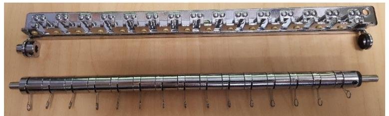
Next, you will want to use a long Allen wrench or long thin screw driver or bar of some sort. When you slide the pieces off the assembly, you want to keep them together as best as possible to make it easier to put back on the assembly. You can grab where the 6th spring is on the assembly and pull it off to the right onto the bar/screw driver/Allen wrench.
