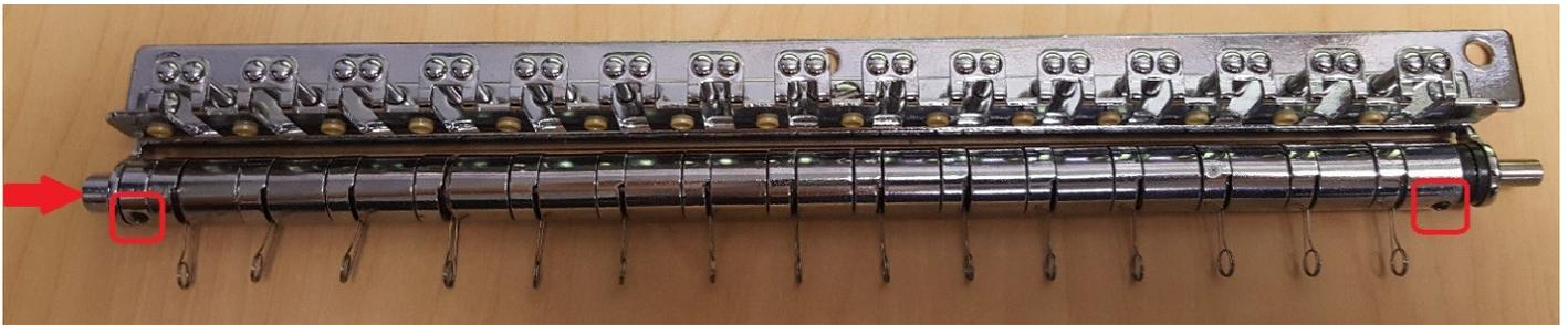
Make sure you can move the take up lever all the way up and all the way down before putting the assembly back on the machine. If all good, put back on the machine and thread everything back up. If it doesn't move all the up like it did, you will need to loosen the set screws and adjust the spring lever.
