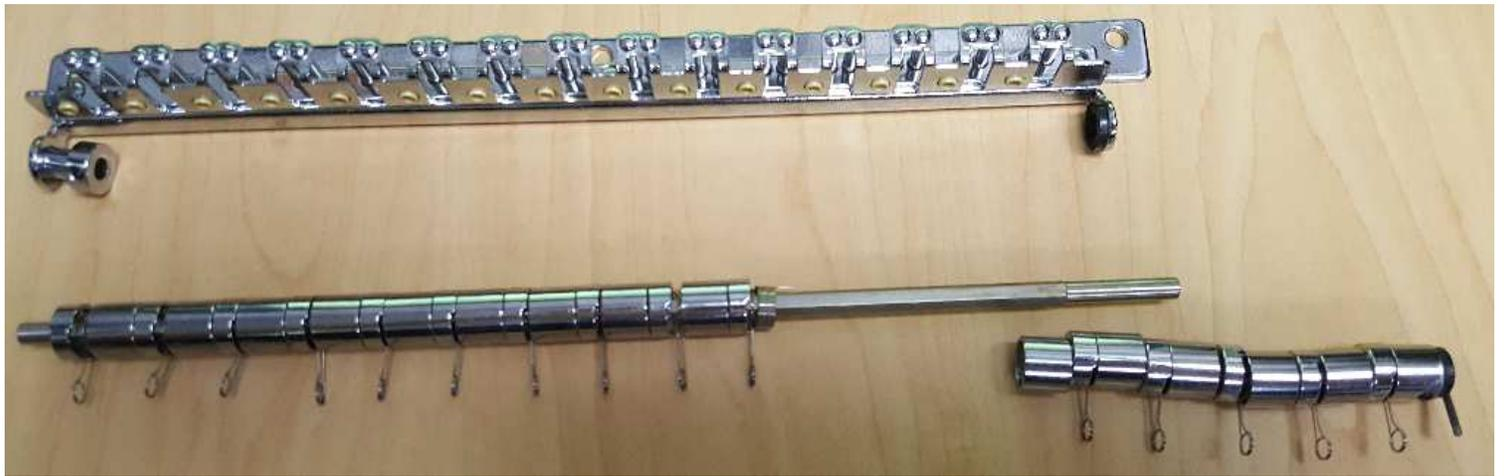
Remove the 6th (broken spring) and replace with the new spring in to the thick metal holder as shown below. Making sure to place the end of the spring's coil in to the hole on the metal cylinder.
