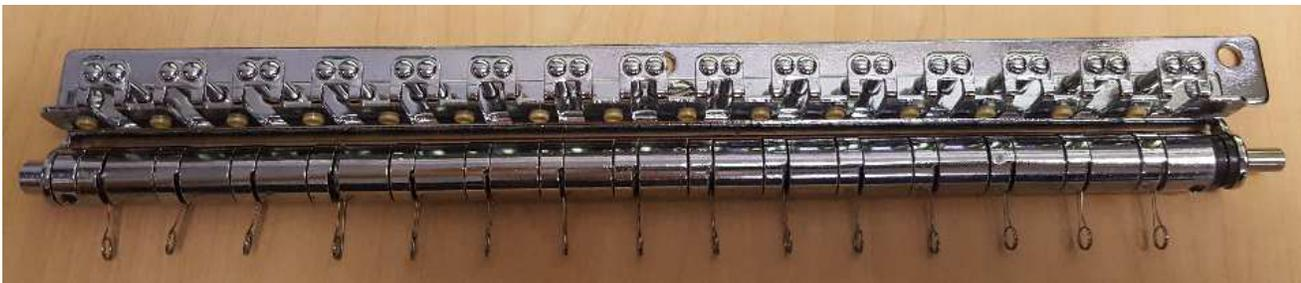
Push the bar on the left to the right until the 2 rubber washers are pushed against each other and hold in place while you tighten down the two Allen screws. Then, place the spring back on and spring lever on the far right, pushing it snugly to the left and tighten down the Allen set screw. With the springs in the down position, your spring lever should be facing down as well.
