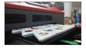
3. Pay close attention to the highest point of the media placed in the machine. Ideally, the media should lay as flat and as even as possible.
