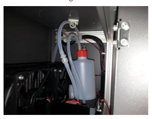
Reach in and lift the reservoir bottle from its location, you may need to angle the bottle to aid in the removal. Bring bottle out as shown below.
