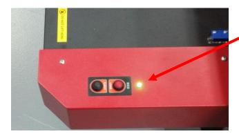
Green LED illuminated indicates bed/media has loaded properly and print data can now be sent to the printer
