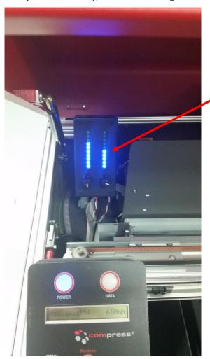
The UV lamp intensity controller can be seen here.
