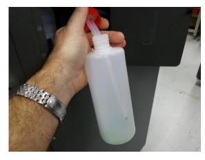
You will notice a green solution in the bottle, this is anti freeze, simply fill the bottle ¾ full with distilled water, reattach the lid and then return bottle to the original location.
