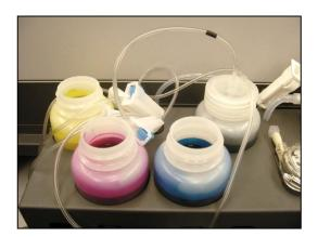
3- Take note of the coloured band on each of the colour ink lines, and match this to the ink in each of the containers when screwing the containers back in to the lids. To screw the containers to the lids, simply hold the lid firmly and screw the container up into the lid.
