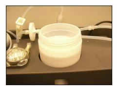
4. Now screw the container back up to the lid. To do this simply hold the lid firmly and screw the container up into the lid. Double check that all tube clamps are in the open position and all connectors are firmly joined.
