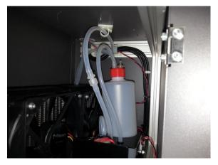
Reach in and lift the reservoir bottle from its location, you may need to angle the bottle to aid in the removal. Bring bottle out as shown below.
