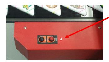
Red LED illuminated indicates print bed/media is not loaded, ensuring correct beam protection is set press the load button to load the bed/media
