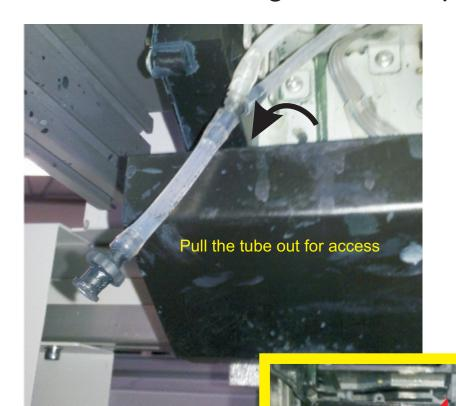
The tube has a connector that can connect directly to your syringe. You can apply flushing solution to your capping station and then use the syringe to draw the flush through the capping station.
