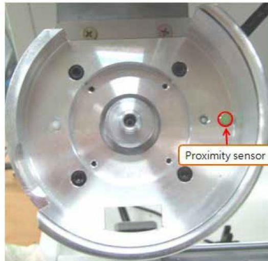
Sensor that detects the Sensor pin.
