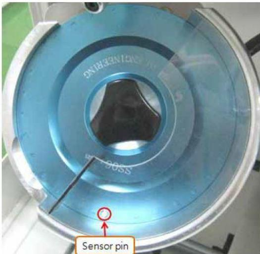
Find the Sensor pin on your Parts Feeder plate and ensure that it is flush with the surface of the plate.
