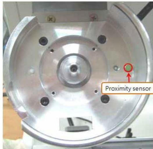
Sensor that detects the Sensor pin.
