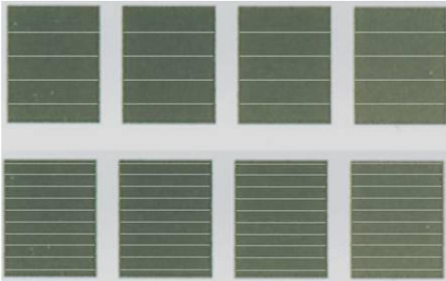
The first row uses two head passes, which produces more visible banding than the four head passes used in the second row. (In this example, the image has been adjusted to make the banding more visible)
