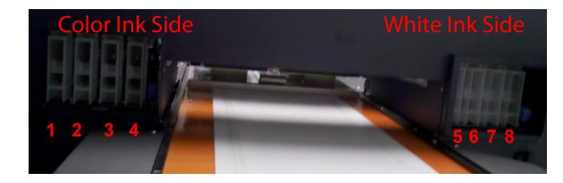
If a cartridge indicates that it is empty on the control panel, use these images to reset the corresponding dummy cartridge.
