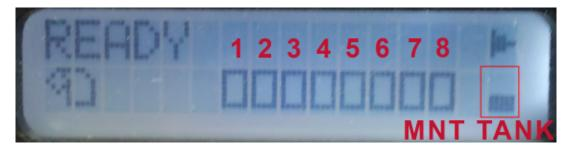
The cartridges indicated on the control panel display of the VIPER are displayed OPPOSITE of the actual dummy cartridge placement.
