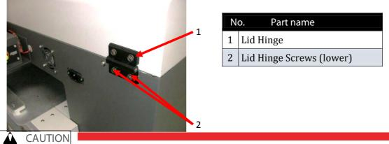
The removal of the top cover (lid) of the M series printers requires two persons: one to hold the lid open during the disconnection of the gus struts, and one at each side of the lid during removal. Injury or damage to the printer may occur if this process is attempted by only one person.
