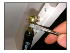
8. Remove the two screws from the lower section of each hinge (left and right hand sides of the rear of the printer) and carefully lift the lid off.
