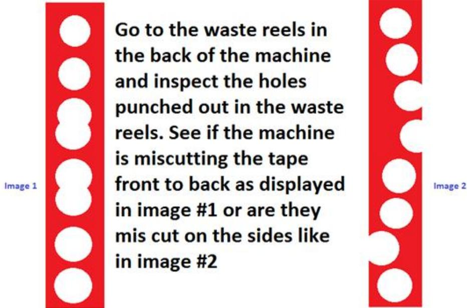
If spangle tape is mis-cutting side to side, check to ensure the Plastic guides are inserted straight and that the spangle tape is correctly interfacing with the guides to disallow the spangle from moving side to side which will cause the spangle tape to be cut from its side.
