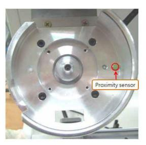
Sensor that detects the Sensor pin.
