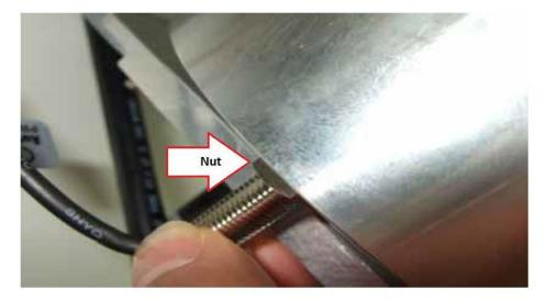
PF Sensor as seen from the rear of the hopper. As you can see it is threaded just like a screw would be, at the top is a nut that holds the sensors position. If this nut is loose then it is possible that the sensor is now slightly too far away from the sensors pin in the plate and it cannot detect it.
