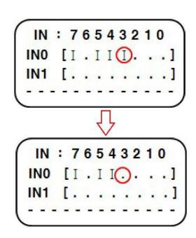
If the "I" does not go out then we need to check to ensure the sensor pin is flush with the side of the plate you are working from (Rhinestone side or Nail head side). If it is and the "I" still does not go out, then we need to bring the sensor up slightly closer so the sensor detects the pin.
